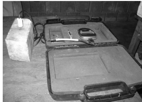
Figure 3. KD2 thermal analyzer probe in a drilled hole inside a sample slab
